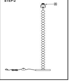
Place Lamp Shade (C) onto the socket and secure by screwing Uno Ring (A) back onto socket clockwise until secured. Remove any plastic wrapping on Lamp Shade (C) before use.
