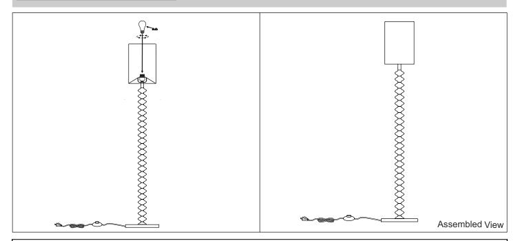
Insert Bulb (not included) into the socket and rotate it in clockwise to secure. Restore power to the circuit at this time and check for proper lighting operation. Assembly is now complete and the product is ready for use.
